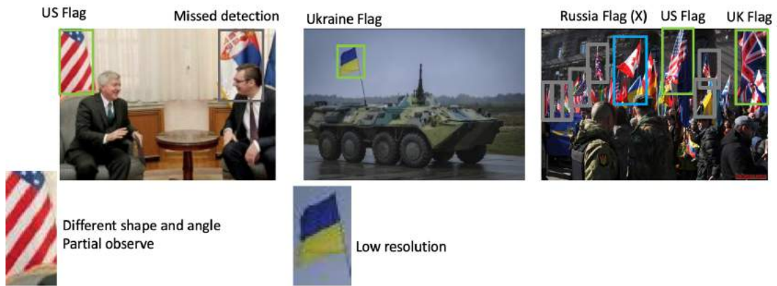
Figure 3: Example flag recognition results. Green represents correct prediction, blue represents wrong prediction, and grey represents missed detection by Faster R-CNN.
